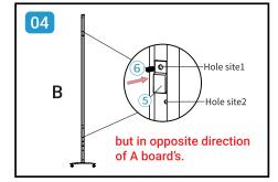
Fix the jointing hook devices (⑤) on the side frame of B board, but in opposite direction of A board's.
