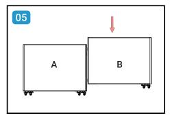
Lock the jointing hook devices of B board downward to the hook devices of A board.
