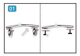
Install the castors(③) on the bottom of the foot cross-bar (②). Two way options: with castors (③), or with foot pad (④)
