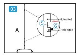
Fix the jointing hook device (⑤) on the side frame of A board by set screw M6x18mm (⑥). Total 3 pieces of jointing hook devices need to two on.
