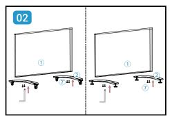
Connect the foot cross-bar(②) to the board by the mounting bolt M8x20mm (⑦)
