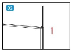
Open the corner cap, pull out the splicing edge sealing strip.
